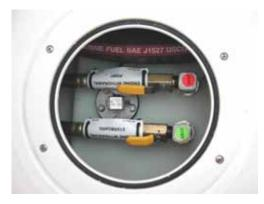
**Fuel Valves Forward Tank (Typical)**
