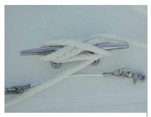
**Anchor Line Secured to Cleat**
