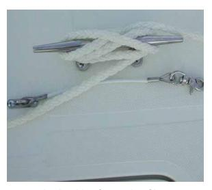
**Anchor Line Secured to Cleat**
