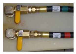
**Fuel Tank Shut Off Valves**
