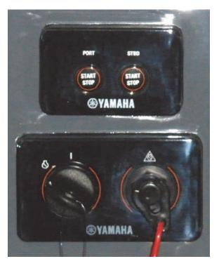
**Engine Stop Switch Lanyard (Typical)**
