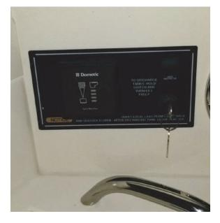
The indicators on this panel display the holding tank level and also includes the holding tank overboard discharge macerator switch. The macerator switch can only be activated when the key switch is fully turned. Refer to Head Compartment of the Interior Equipment.
