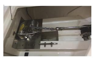
**Anchor Line Secured Using Cable**
