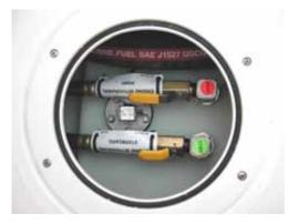
**Fuel Valves Forward Tank (Typical)**
