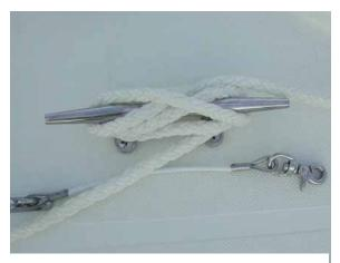
**Anchor Line Secured to Cleat**
