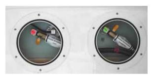
**Fuel Valves Aft Tank (Typical)**
