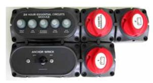
Battery Switches and Main Breakers Twin Engines (typical)
