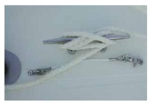
**Anchor Line Secured to Cleat**
