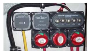
Battery Switches and Main Breakers Single Engines (typical)
