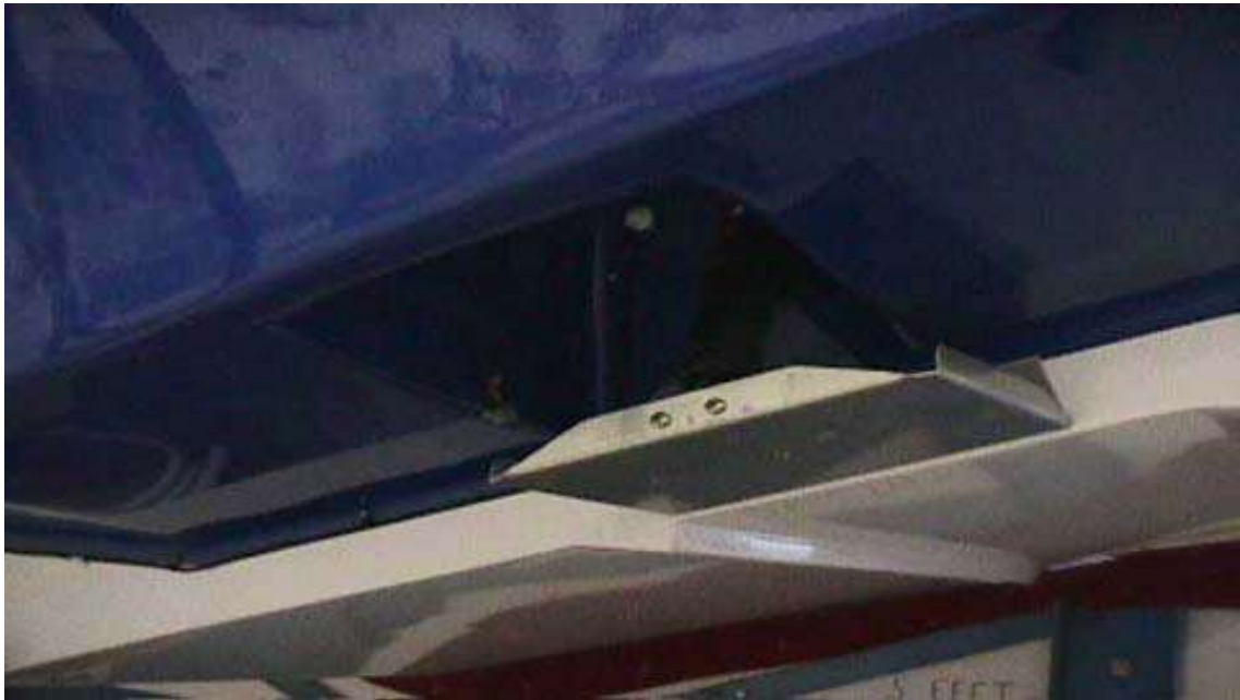
Fig. 3 trim tabs, shown in the up position
