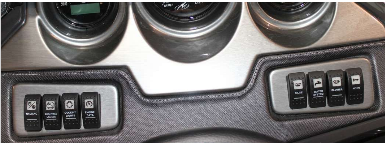
Helm Switch Panels 214SS/218SS & 234SS/238SS
