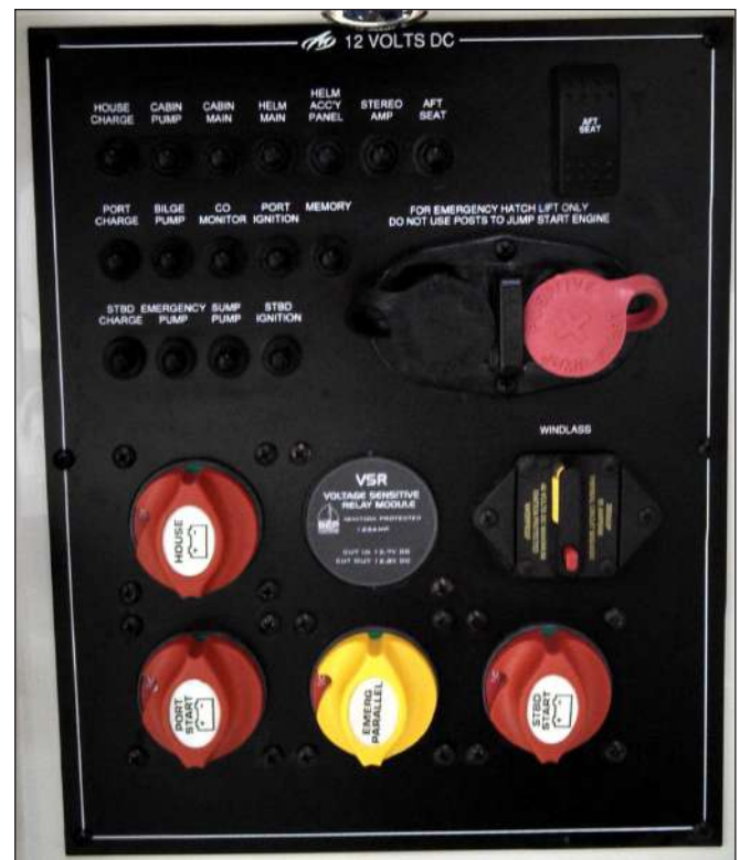
328SS Battery Switch Panel, Circuit Protection & Switches
