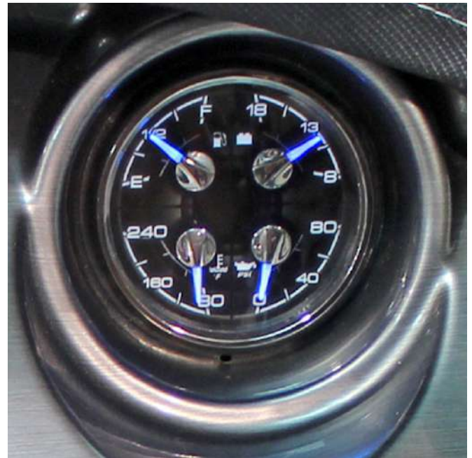
Typical Backlit Multi Gauge Fuel Level, Engine Temperature, Voltage & Oil Pressure
