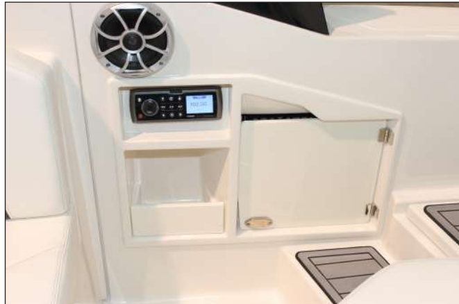
288SS Transom/Battery Switch Panel Door Door Enclosing Battery Switch Panel
