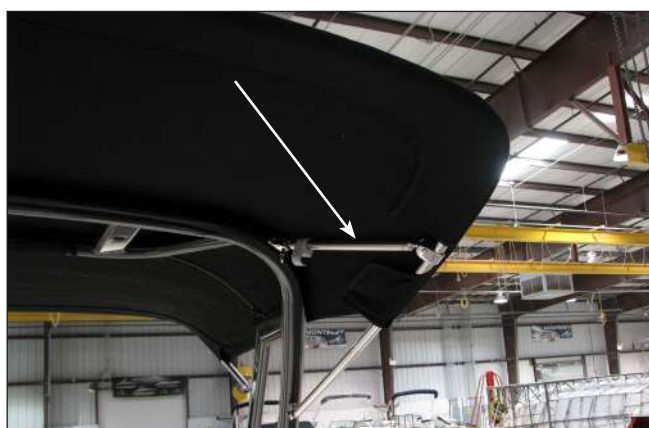
Front Top Open & Supported With Stanchion
