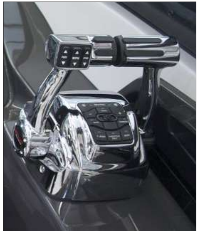
Mer cruiser Twin Engine Electronic Controls
