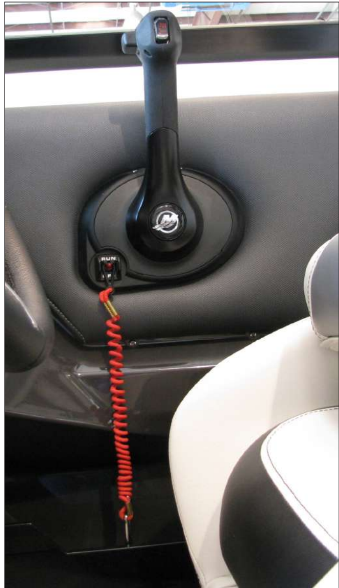
Mercruiser Control Emergency Stop Switch & Lanyard
