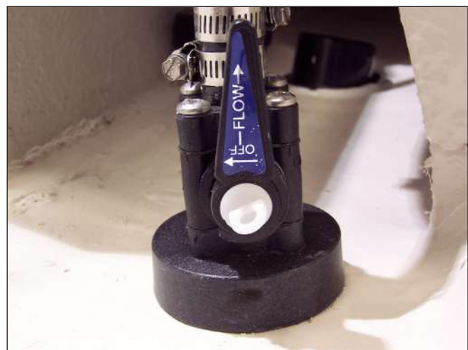
Air Conditioner Seacock (Thru-Hull Valve)
