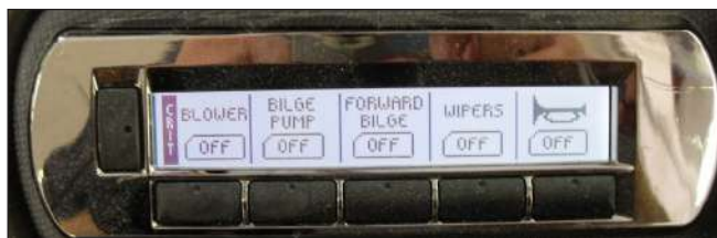
Critical Page - Digital Switch Panel
