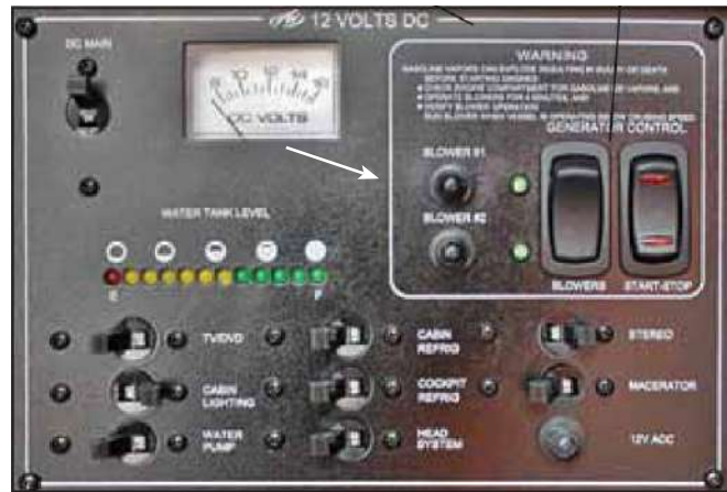
Optional Generator Control Panel In Cabin DC Panel
