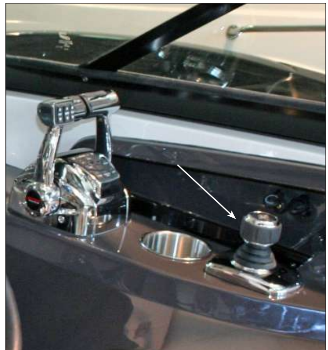
Typical Mercruiser DTS Joystick Control
