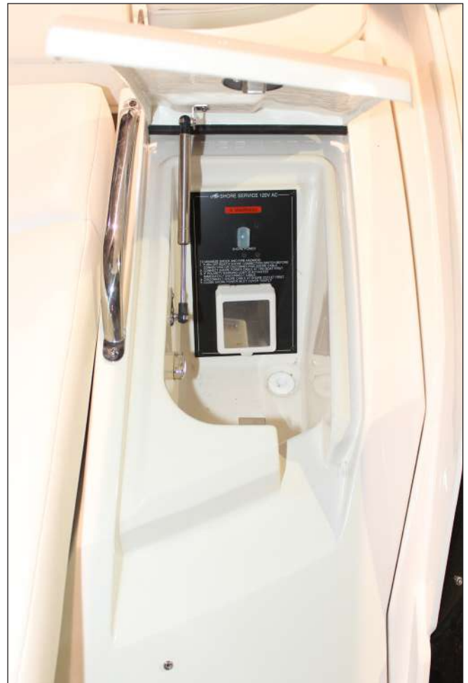
328SS Shore Power Inlet Panel
