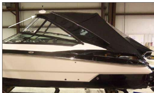
328SS Arch Canvas & Connectors Installed Note that front clear connection attaches directly to arch
