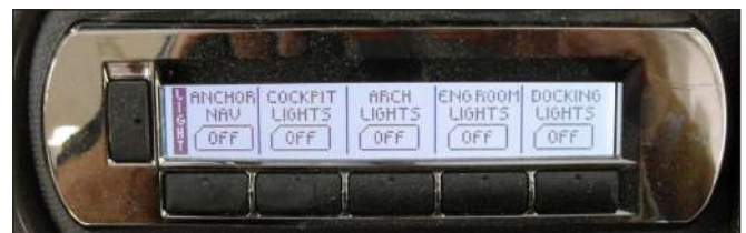
Lights Page - Digital Switch Panel
