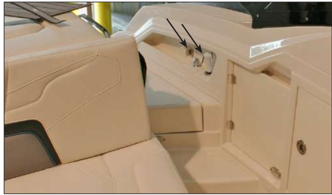
328SS Cockpit Shower Head & Shower Water Connection
