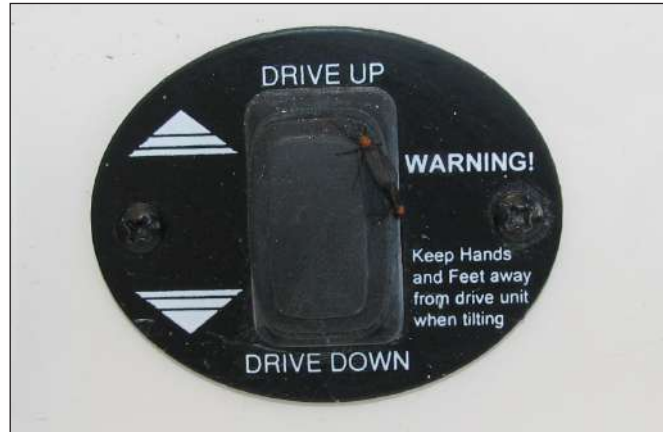
Typical Outdrive Tilt Switch Near Transom Door
