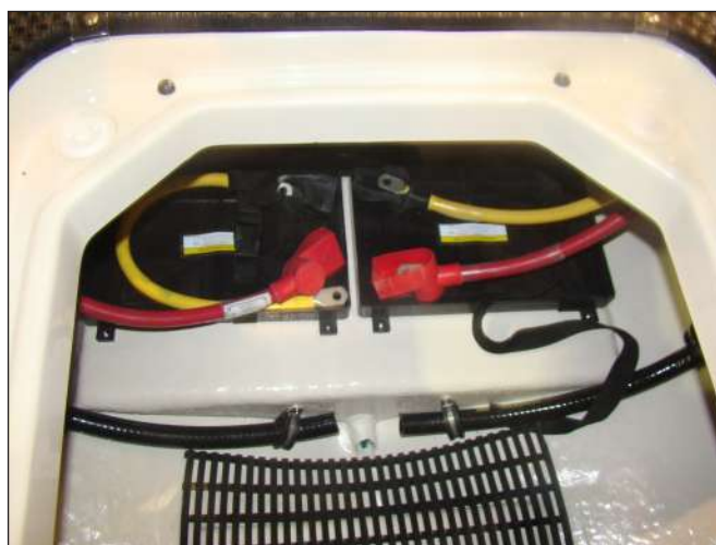
In-Floor Storage Compartment Battery Mounting Location 214SS/218SS & 234SS/238SS
