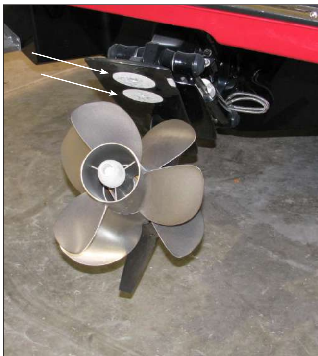
Typical Mercruiser Outdrive Anodes
