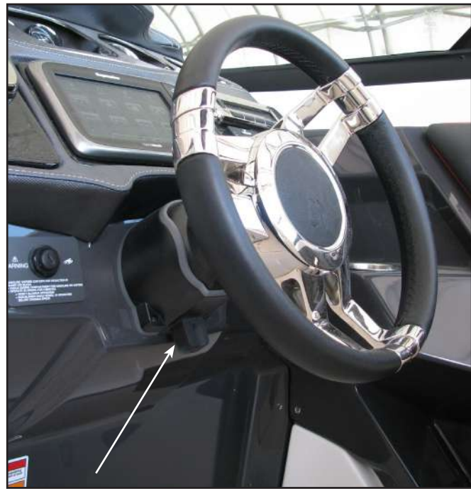
Tilt Steering Wheel & Tilt Release Lever
