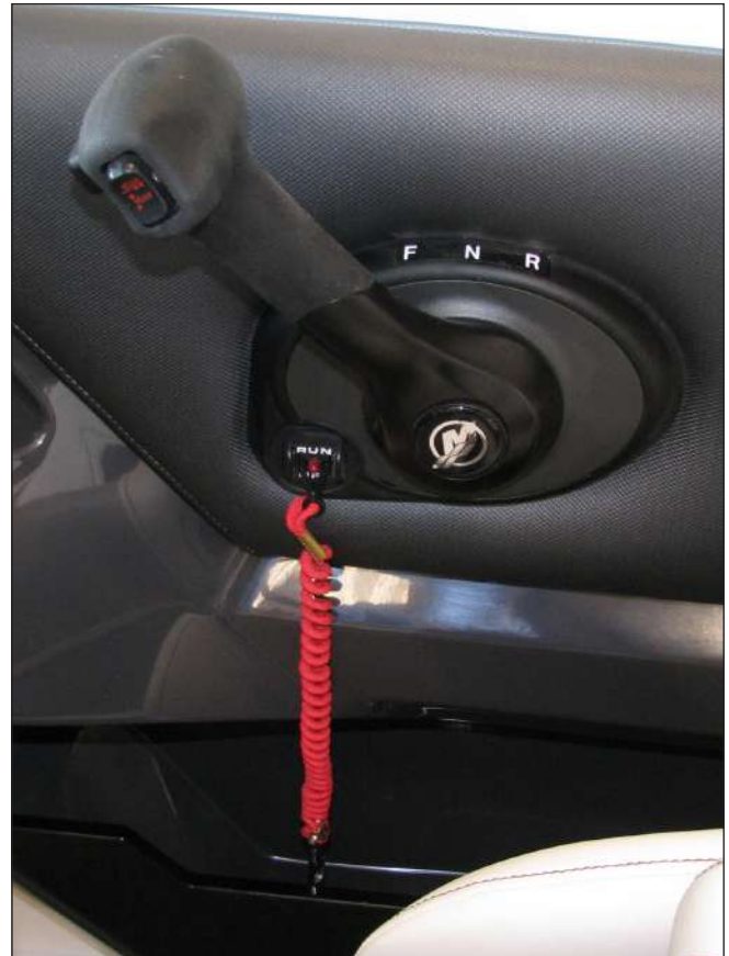
Mercruiser Side Mount Cable Control & Stop Switch
