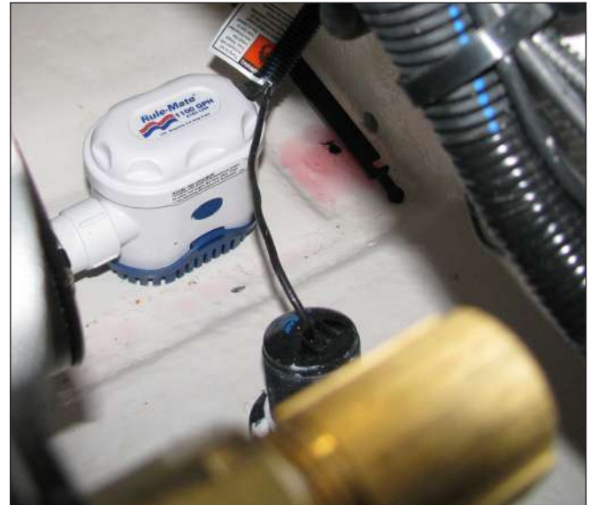
Aft Automatic Bilge Pump 214SS/218SS/234SS/238SS/268SS/288SS
