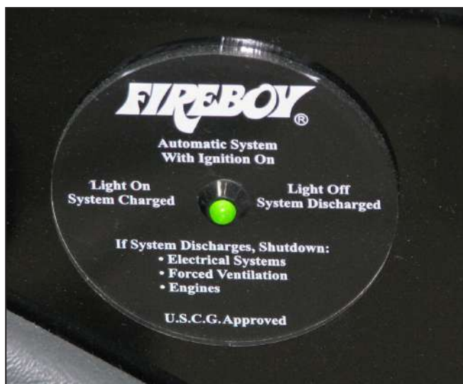
Fire Extinguisher Panel In Helm
