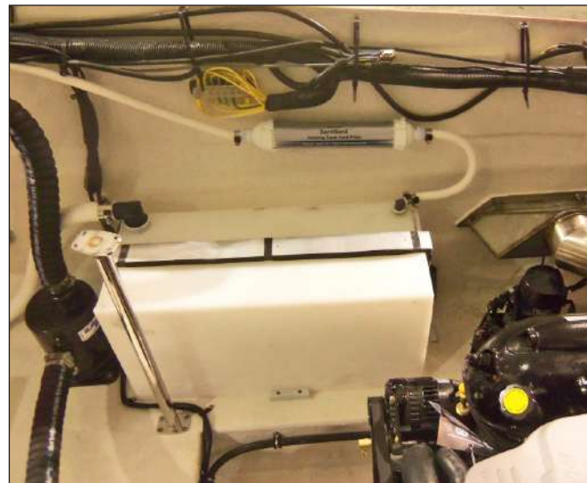
328SS Holding Tank & Charcoal Filter
