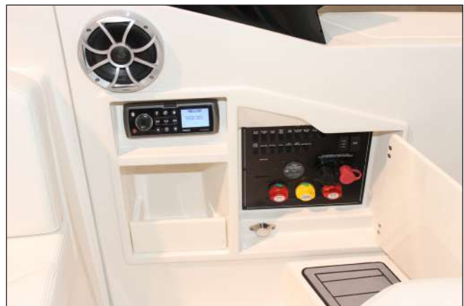
288SS Transom/Battery Switch Panel Door Door In Transom Door Position Closing Off Swim Platform Walkway
