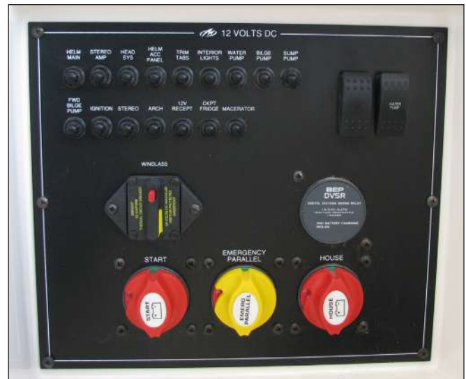
288SS Dual Battery Switch Panel & Circuit Protection
