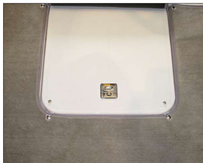
Typical Twist Lock Latch - Latched With Handle Folded Flush
