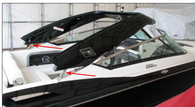
Fiberglass Electric Folding Arch & Actuators
