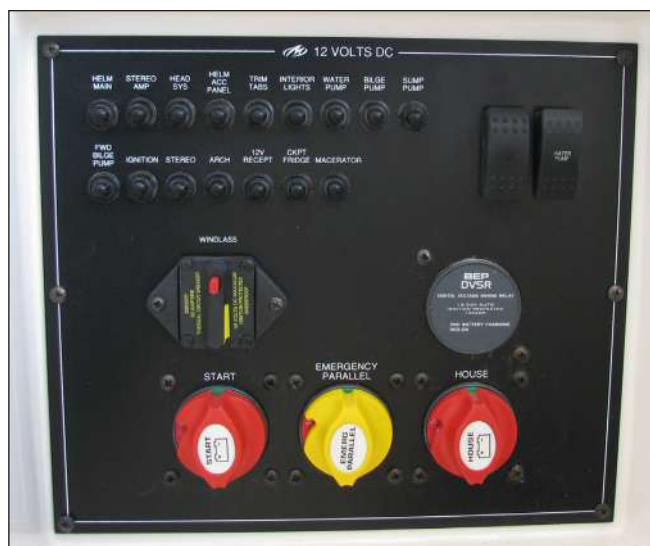
288SS Battery Switch Panel, Circuit Protection & Switches
