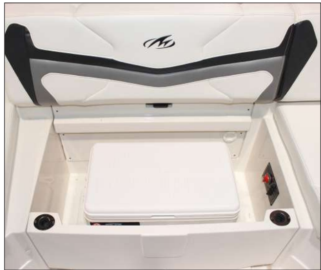
Cooler/Battery Switch/Fire Port Compartment 214SS/218SS & 234SS/238SS
