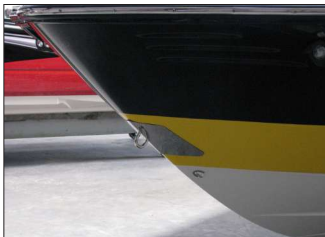
Typical Rope Locker Drain
