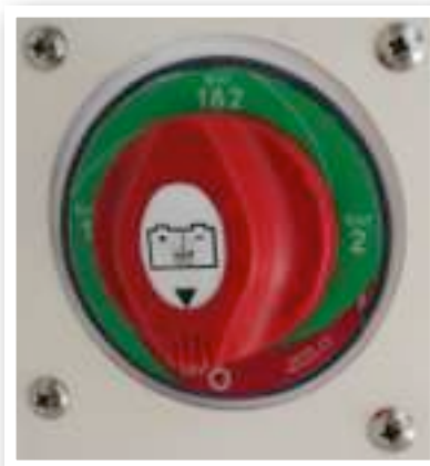
Battery Switch, Shown in the "Off" Position
