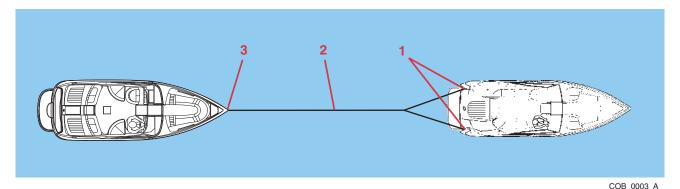
Adjust the tow line to match wave action. Keep the boats on the crest or in the trough of the waves at the same time. In protected, calm waters, shorten the line for better handling. Tow at moderate speed, allowing for adverse wind and wave conditions. Have the operator of the towed boat steer with you, if possible.
