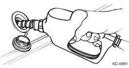
When your boat is equipped with the pop-up fuel filler cap, open by pressing the cap and turning the cap counterclockwise (approximately 10°); remove cap.
