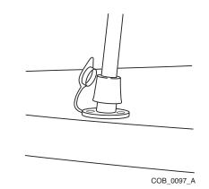
Cap the anchor light socket when the anchor light is removed.
