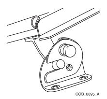
To close the windshield, release the locking mechanism by pulling the forward-facing button. Swing the windshield into place.
