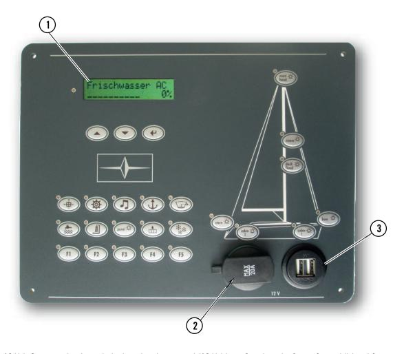
The 12 Volt Systems circuits switched on the above panel (12 Volt) are fused on the front of an additional fuse panel which is situated, below the switch panel.
