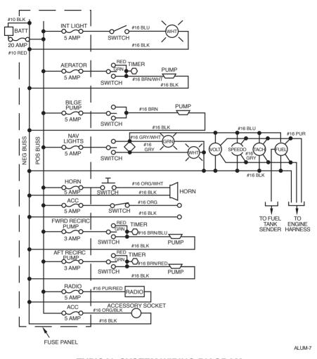
TYPICAL SYSTEM WIRING DIAGRAM
