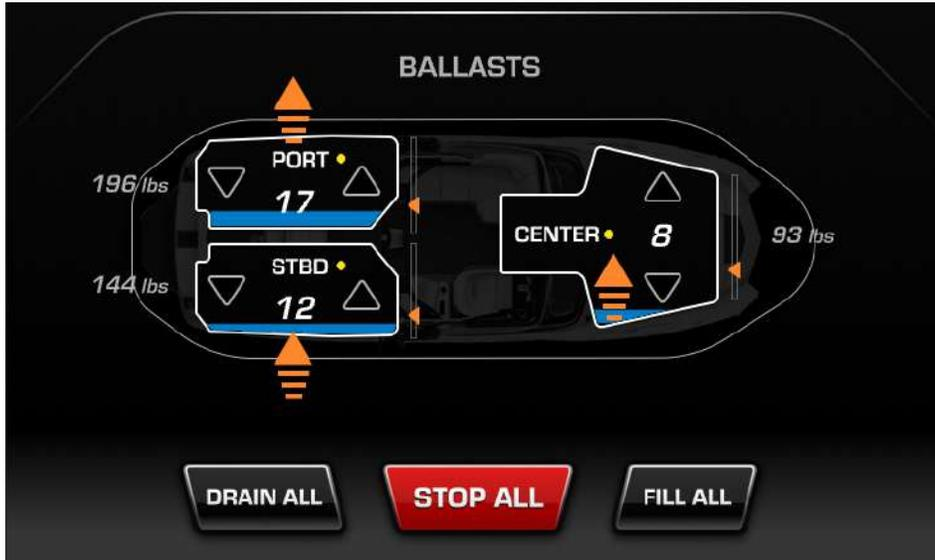
Ballast is used to add displacement to the craft in order to make the waves or wakes larger for specific watersports.
