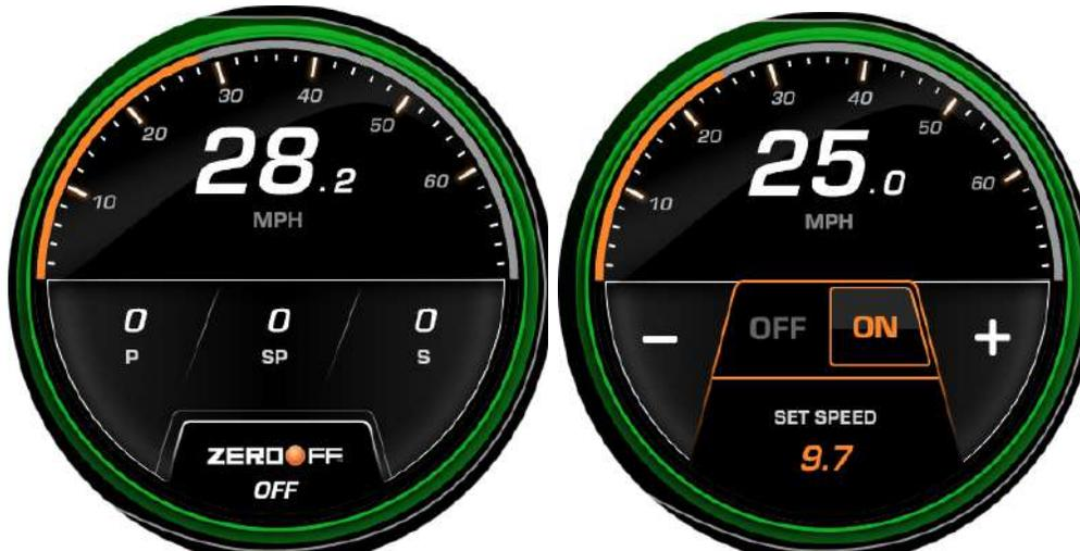
Touch the ZeroOff Off button to turn on the GPS speed control. After a few seconds, the Set Speed controls will appear.
