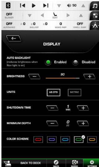
**Auto Backlight:** this automatically dims the brightness when the Navigation light is on.
