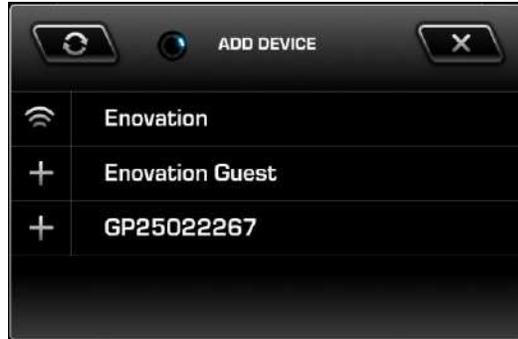
Note: Be sure to set the camera name and password via the GoPro mobile phone application. Open your camera settings and check that Wireless is on and in RC+APP mode.
