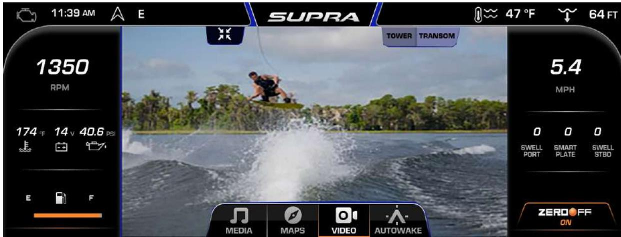
Touch the Tower or Transom button to switch to the alternate video view.
