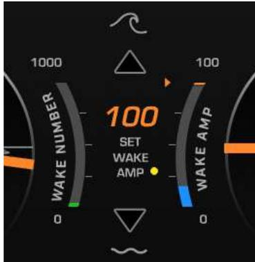
Use this setting to define the amplitude of your wake (0 is mellow and 100 is aggressive). The Wake Amp\* bar will fill (in blue) or empty to the target Wake Amp setting (orange pointer). This blue fill will indicate your total fill level for all ballast.
