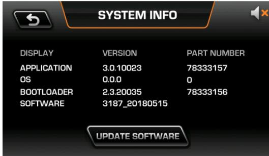
Like the System Information screen in the PV100, this screen provides version and part numbers for the Application, Operating System, Bootloader and Software, along with a way to update the software.
