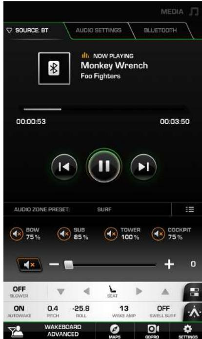
Touching the top tab on the PV1100 display will shift the screen down and this screen will appear.
