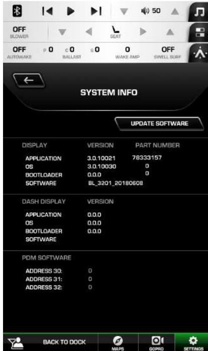
This screen displays the current version and part numbers for the Application, Operating System, Bootloader and Software used on the display, dash display and PDM software.
