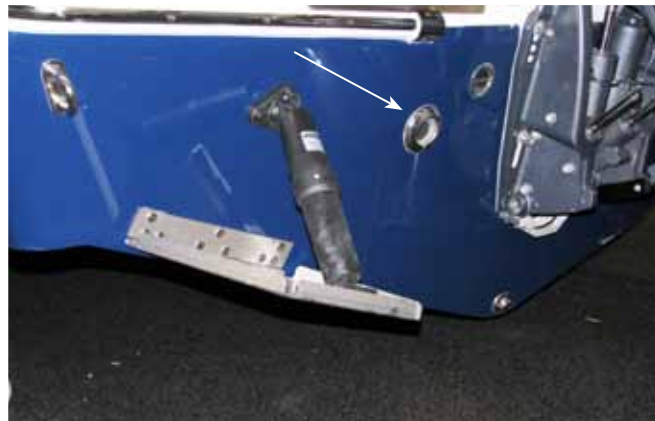
Transom Scupper Drain Check Valve Assembly
