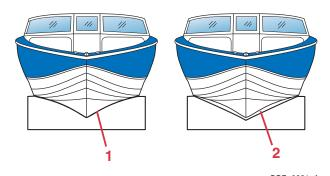
1 - Hull completely on cradle - right
