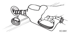
When your boat is equipped with the pop-up fuel filler cap, open by pressing the cap and turning the cap counterclockwise (approximately 10°); remove cap.
