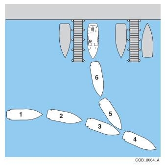
This maneuver is similar to backing an automobile into a garage or parking space. When approaching a slip:
