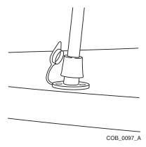
Cap the anchor light socket when the anchor light is removed.
