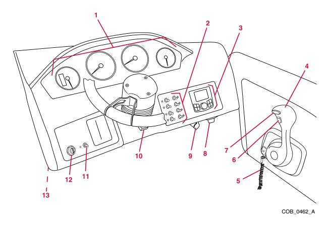
Your Cobalt boat helm will monitor and provide operation of the boat's functions. The gauges are illuminated for night operation.
