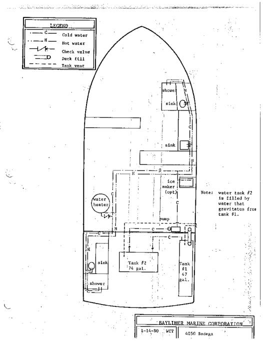
The 110 wolt heating element in the tank will burn up if there is no water in the tank.
